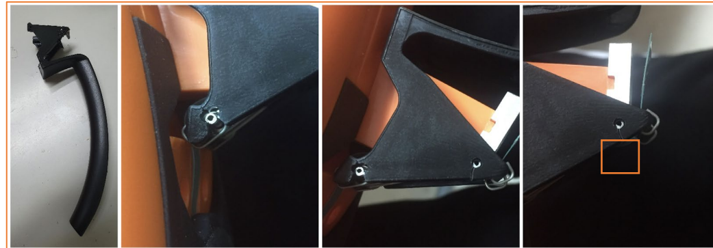
Figure 1: Paddle head fracture points
