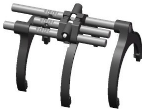
Figure 1: The Structure of lorry's shift mechanism [1]
